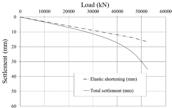
Figure 14 Cemset Pylon Pile head prediction
