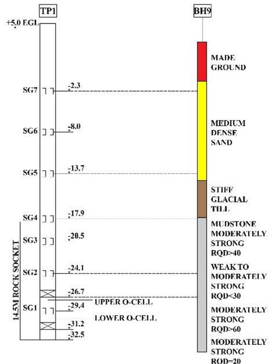
Figure 2. Geology & Instrumentation at Test Pile
