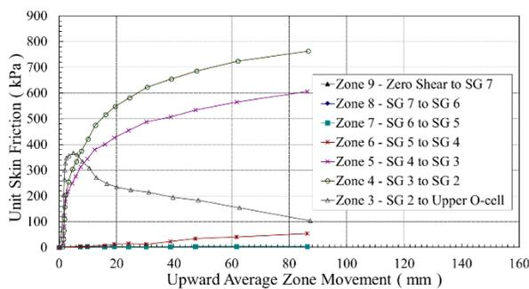
Figure 11 – Mobilised unit skin friction – Stage 2
