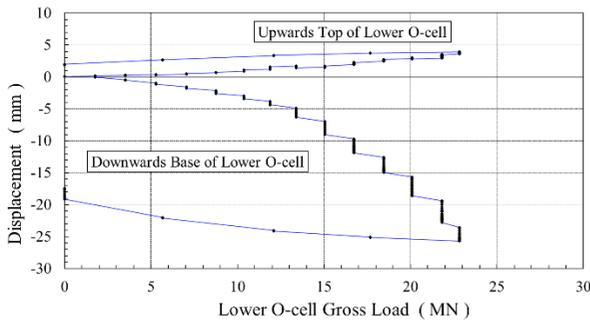
Figure 7- Load displacement of lower O-cell Stage 1
