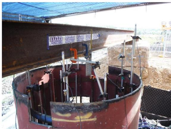
Figure 6 Instruments and reference beam over the test pile head
