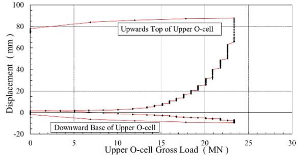
Figure 8 Load displacement of upper O-cell Stage 2
