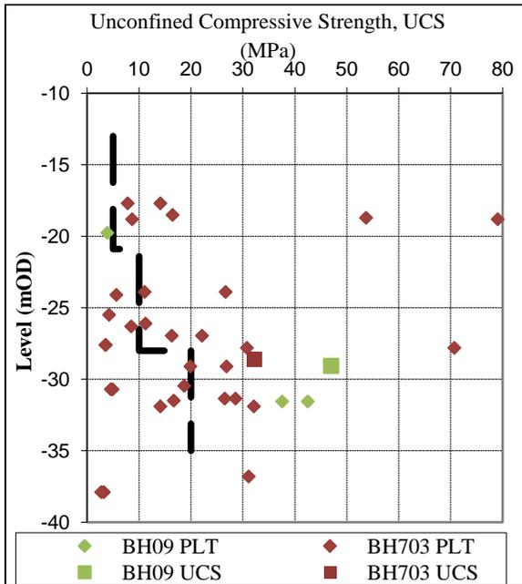
Figure 4 UCS v Level at Preliminary Test Pile
