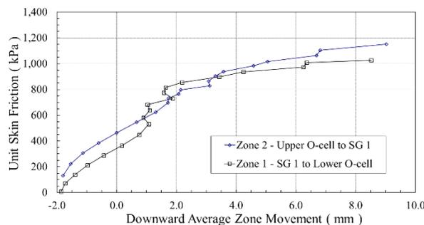
Figure 12 – Mobilised unit skin friction – Stage 2
