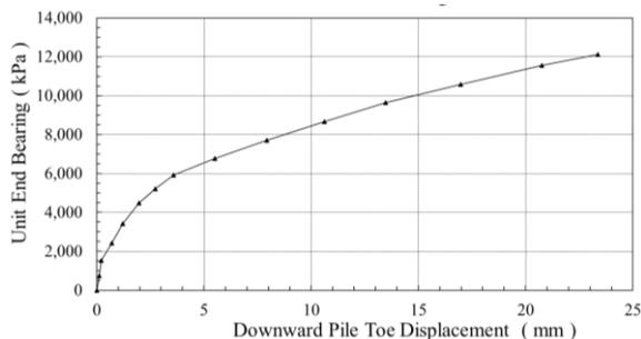
Figure 13 – Mobilised Unit end bearing in Stage 1
